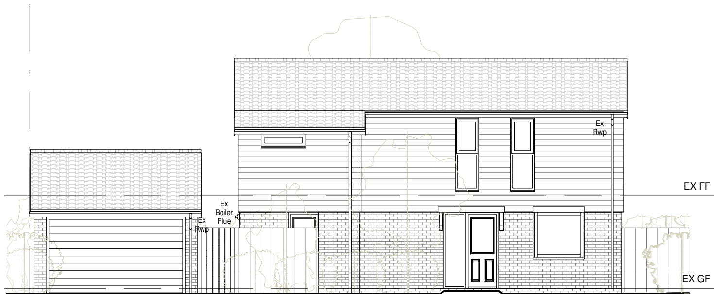
3 Existing South Elevation 1 : 100
