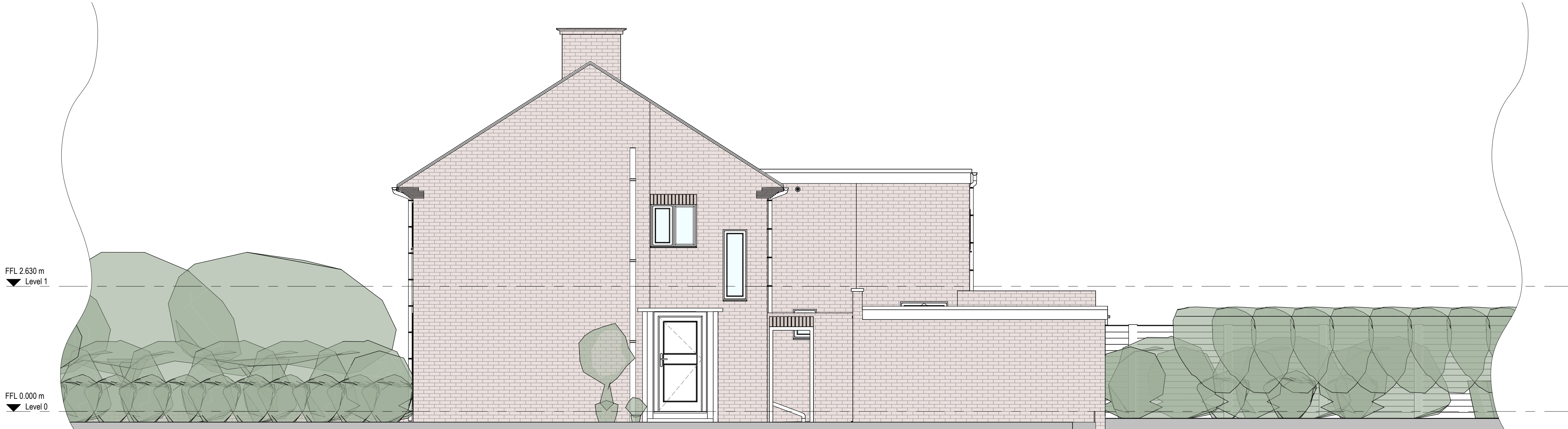
1 Side Elevation as Existing 1 : 50
