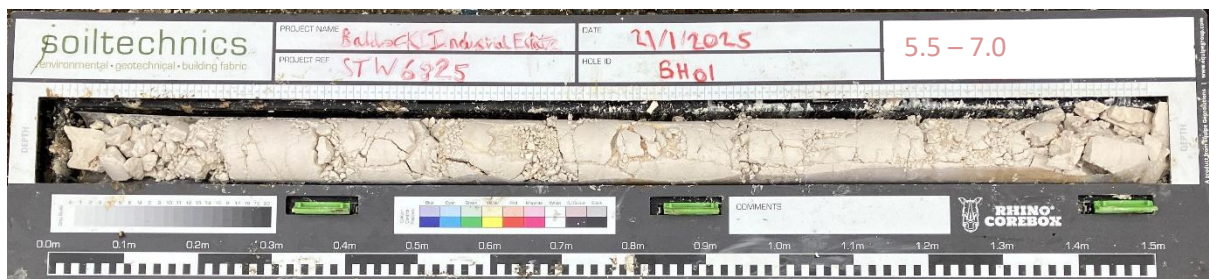
P10: Photograph showing recovery from BH01 between 5.5m and 7.0m
