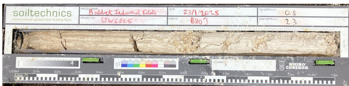
Figure 6-C: Structureless chalk encountered in BH03.
