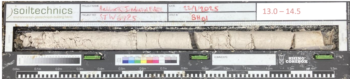
P15: Photograph showing recovery from BH01 between 13.0m and 14.5m
