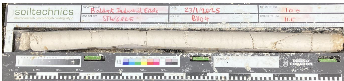
Figure 6-D: Structured chalk encountered in BH04.
