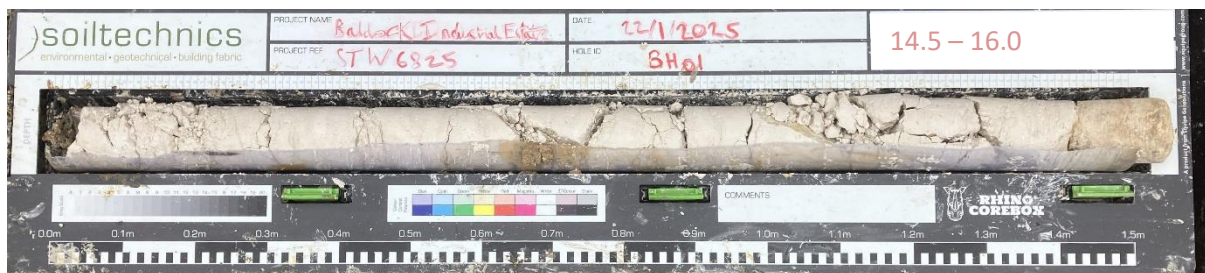
P16: Photograph showing recovery from BH01 between 14.5m and 16.0m
