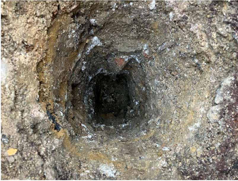
Figure 6-A: Made Ground within the inspection pit at BH02.
