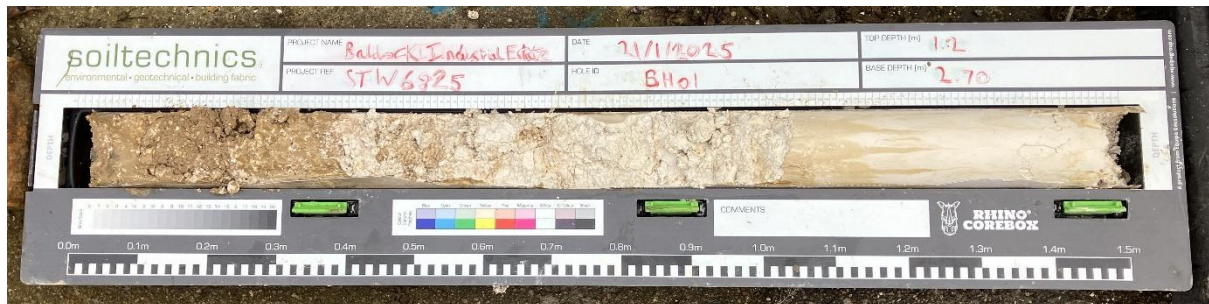
P7: Photograph showing recovery from BH01 between 1.2m and 2.5m
