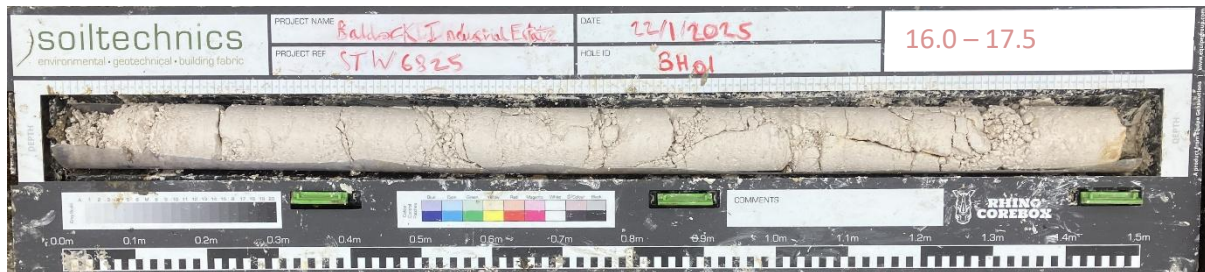
P17: Photograph showing recovery from BH01 between 16.0m and 17.5m
