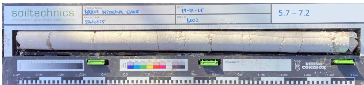
P21: Photograph showing recovery from BH02 between 5.7m and 7.2m
