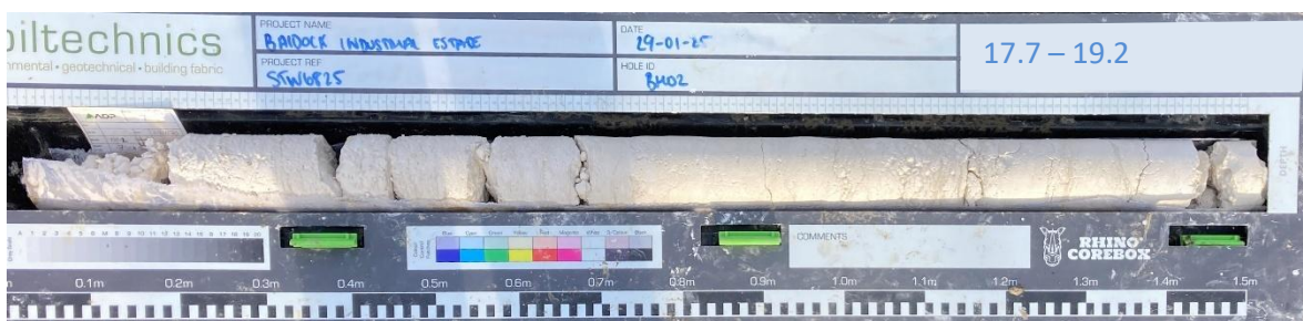
P29: Photograph showing recovery from BH02 between 17.7m and 19.2m
