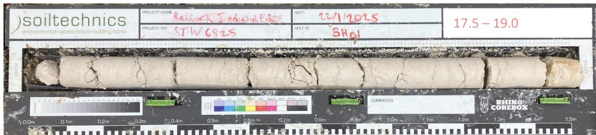
P18: Photograph showing recovery from BH01 between 17.5m and 19.0m
