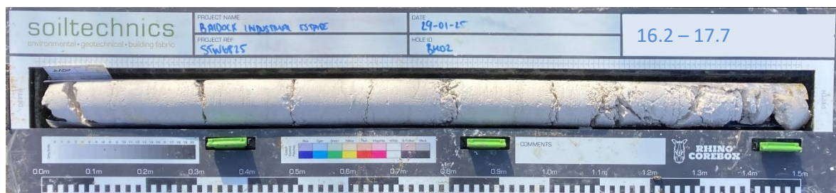
P28: Photograph showing recovery from BH02 between 16.2m and 17.7m
