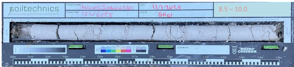
P12: Photograph showing recovery from BH01 between 8.5m and 10.0m
