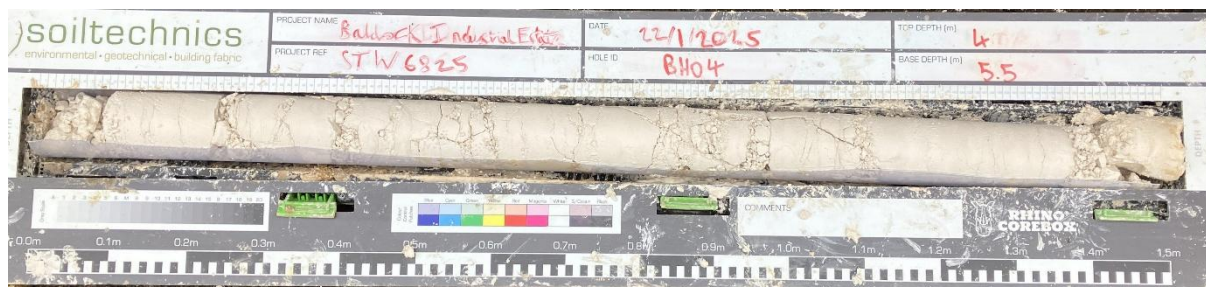
P43: Photograph showing recovery from BH04 between 4.0m and 5.5m
