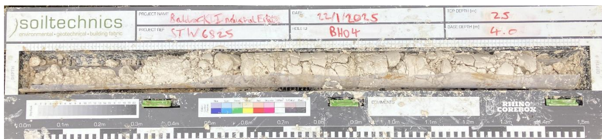
P42: Photograph showing recovery from BH04 between 2.5m and 4.0m
