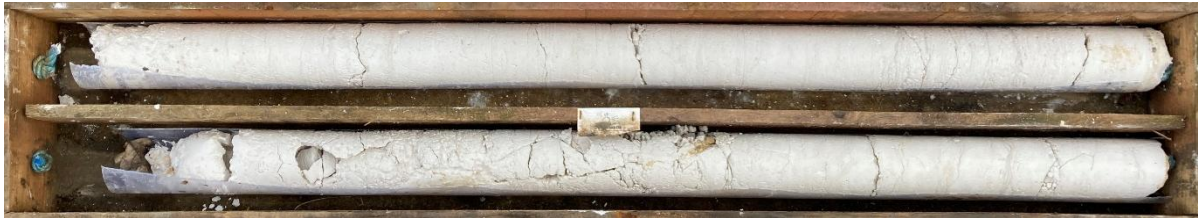
P49: Photograph showing recovery from BH04 between 13.0m and 16.0m
