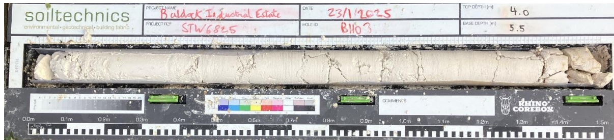
P33: Photograph showing recovery from BH03 between 4.0m and 5.5m
