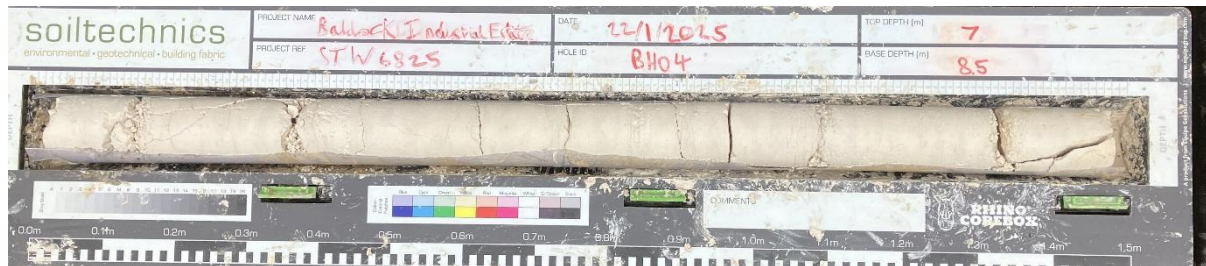
P45: Photograph showing recovery from BH04 between 7.0m and 8.5m
