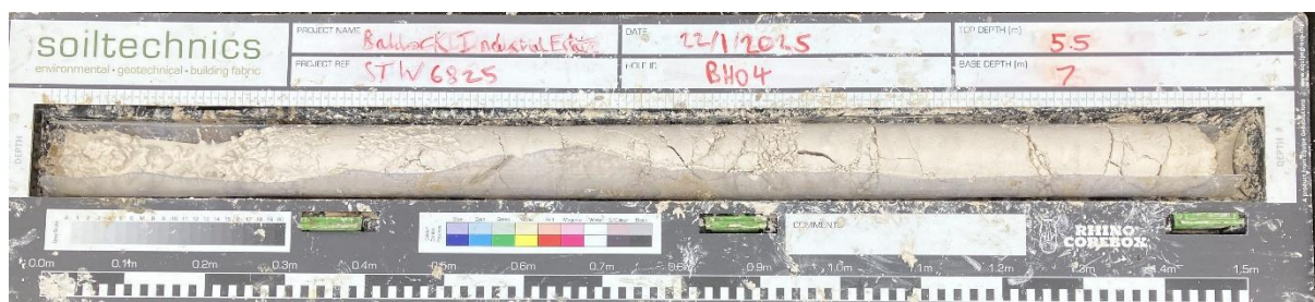
P44: Photograph showing recovery from BH04 between 5.5m and 7.0m
