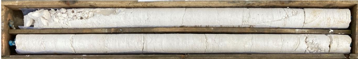
P38: Photograph showing recovery from BH03 between 13.0m and 16.0m
