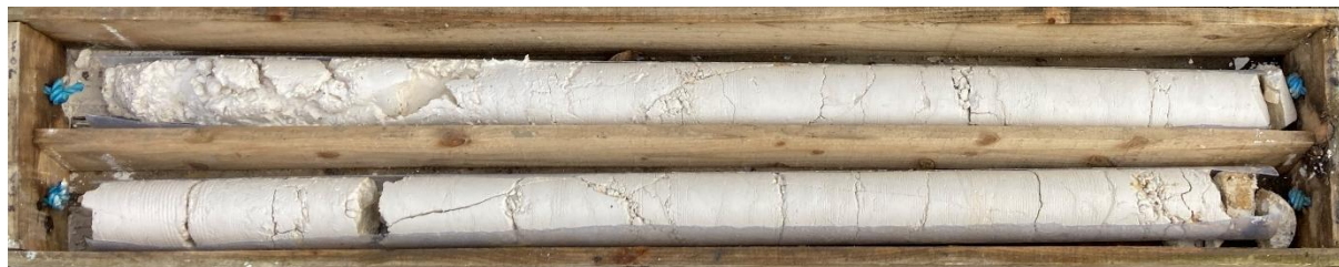
P36: Photograph showing recovery from BH03 between 7.0m and 10.0m
