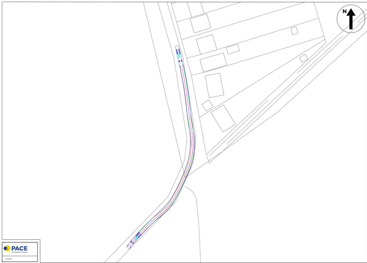
Figure 8.2: Swept path diagram showing vehicles successfully negotiating the bend along Ashwell Road before continuing southwards towards the A507.
