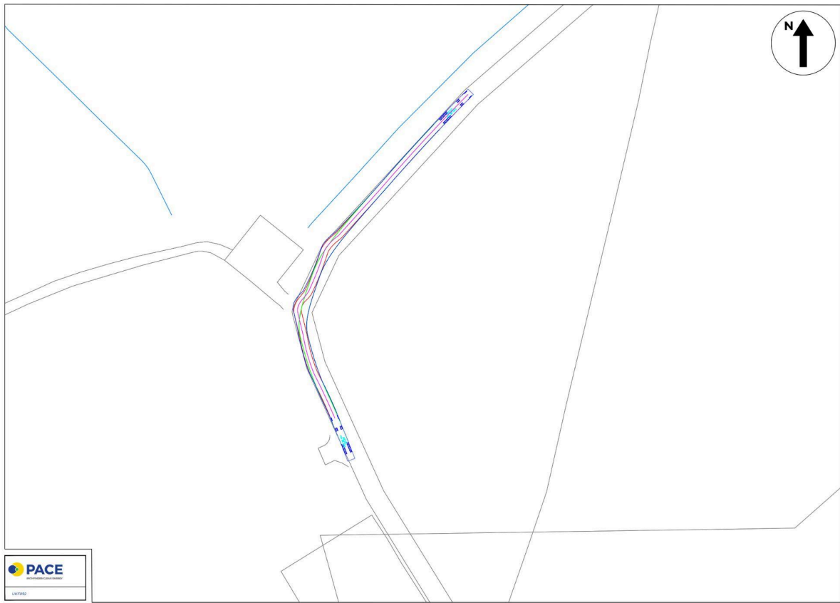
Figure 8.5: Swept path diagram showing vehicles successfully negotiating the bend along Ashwell Road before continuing southwards towards the A507.
