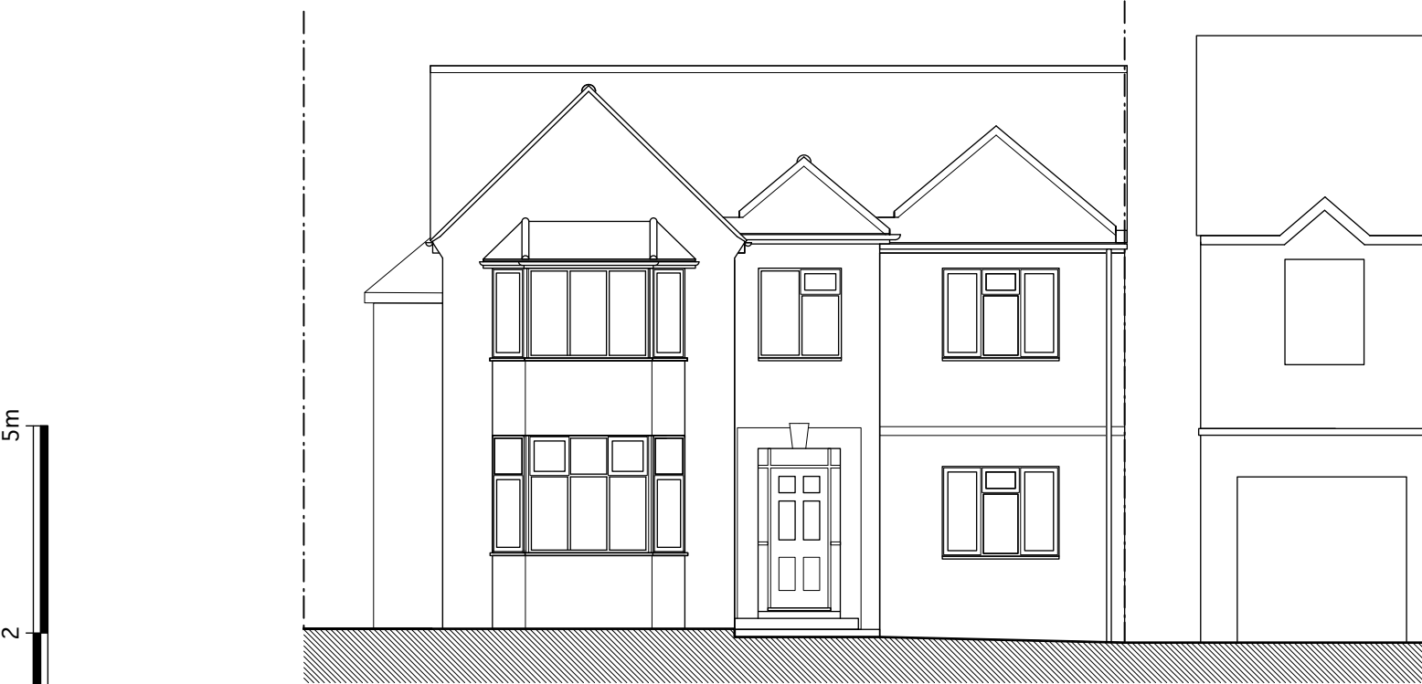
Pre-existing Front Elevation (1:100)
