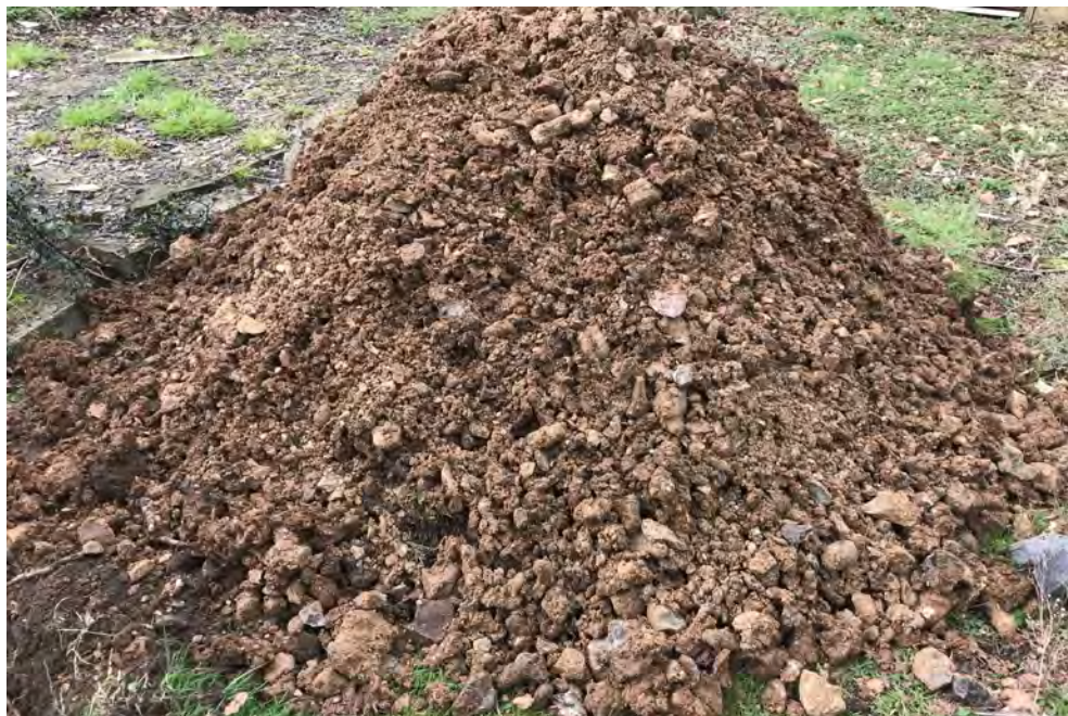
Soil arisings of trial pit TP4
