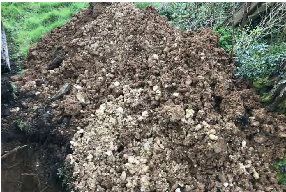
Soil arisings of trial pit TP6
