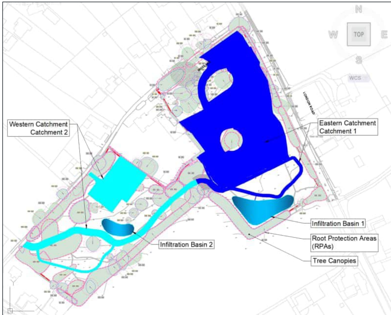
Figure 7-2 - Drainage Catchments and Infiltration Basins
