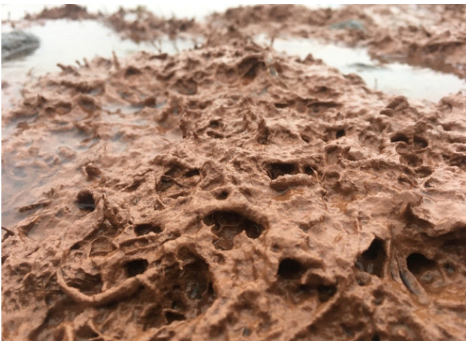
Close up Floc Mat showing accretion of silt
