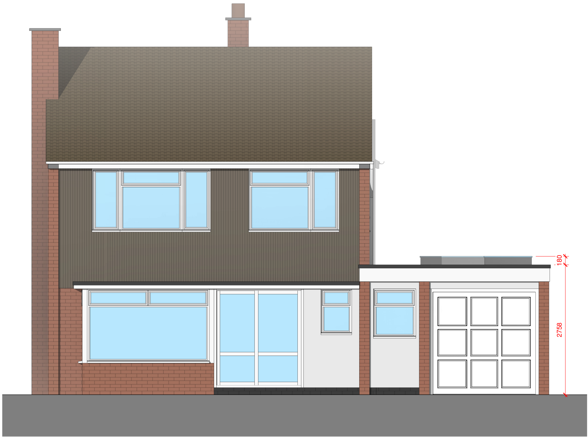
1 Front Elevation - Proposed 1 : 50
