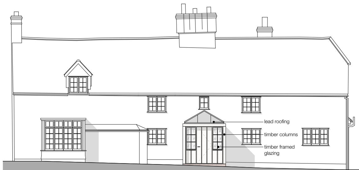
south elevation showing the proposed porch
