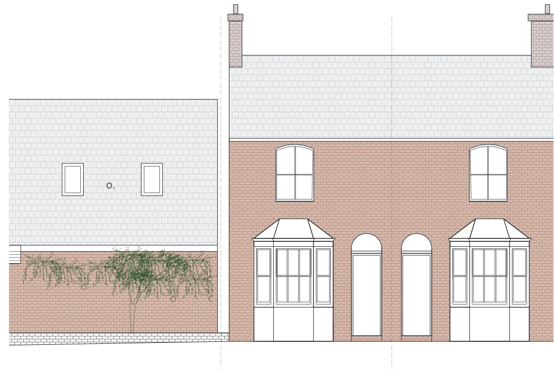
Front North Elevation, Existing 1:50 @ A3
