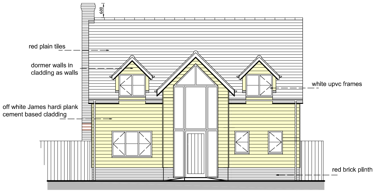
FRONT (EAST) ELEVATION
