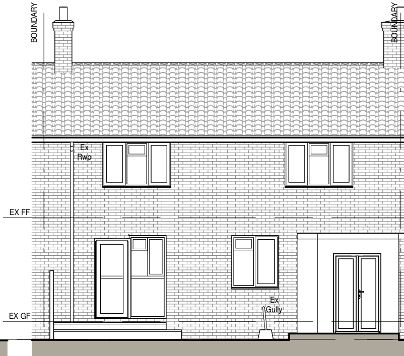
5 Existing South Elevation 1 : 100
