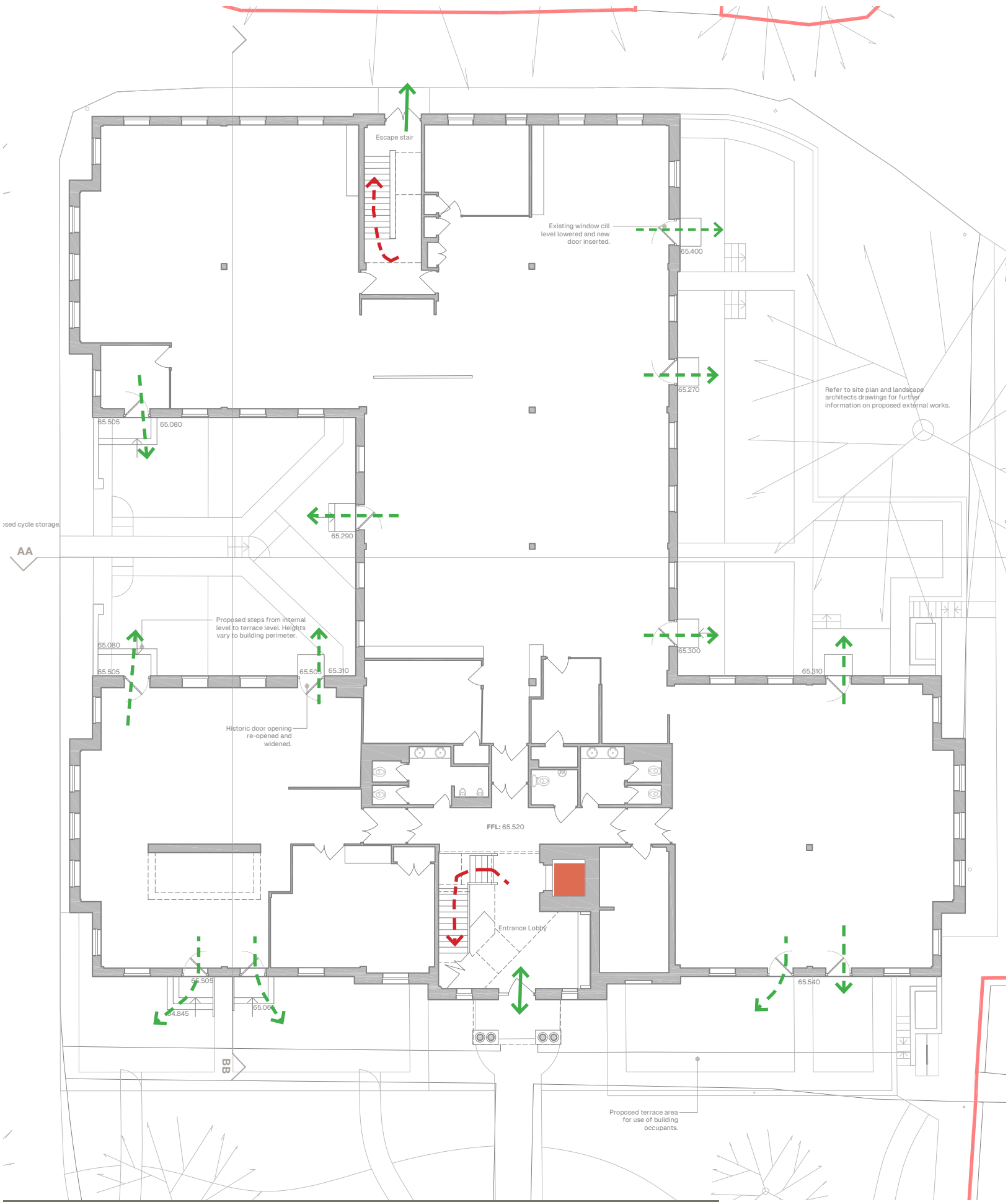
FIGURE 18: GROUND FLOOR ACCESS POINTS
