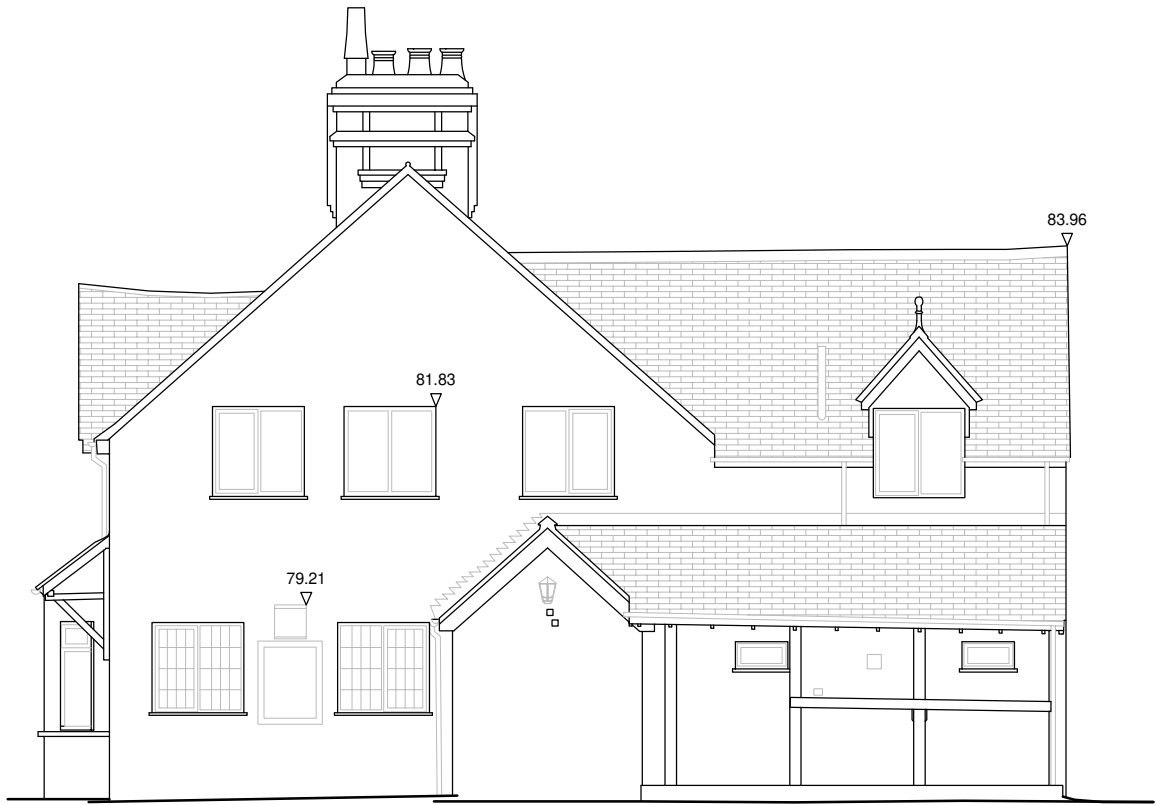
SOUTH ELEVATION Datum 75.00m
