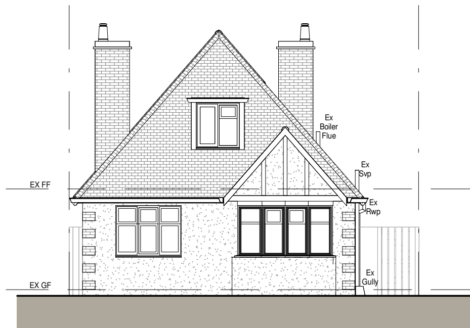
3 Existing North Elevation 1 : 100
