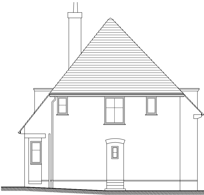
Existing Side Elevation
