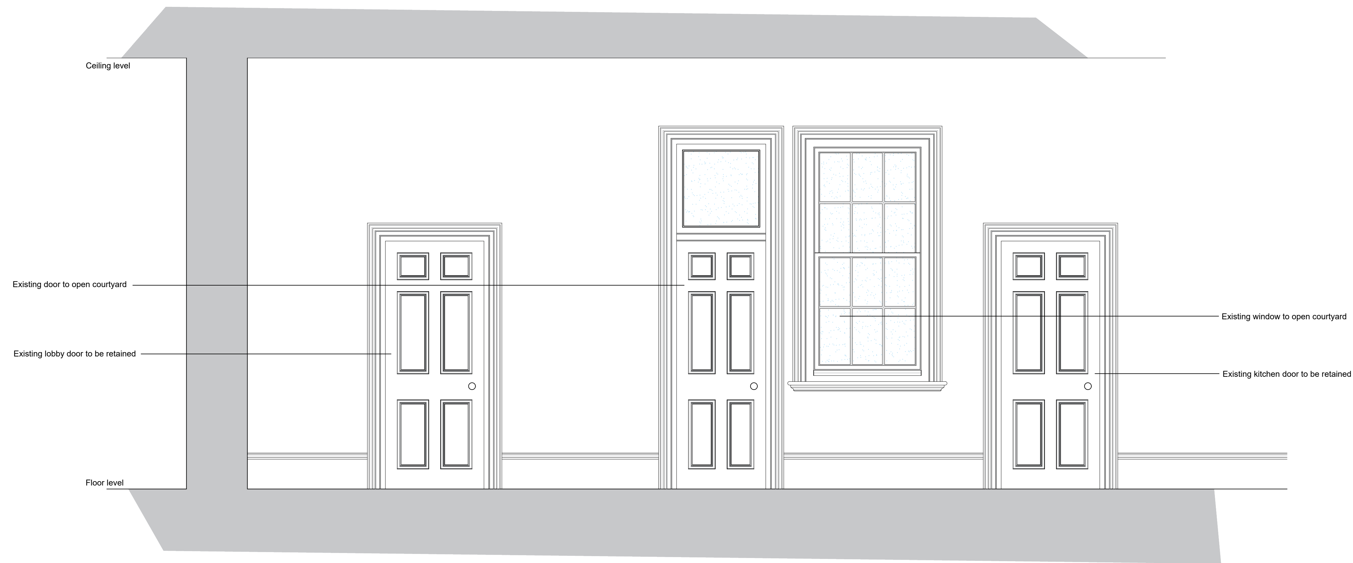
Existing Service Hall Internal Elevation 1:20
