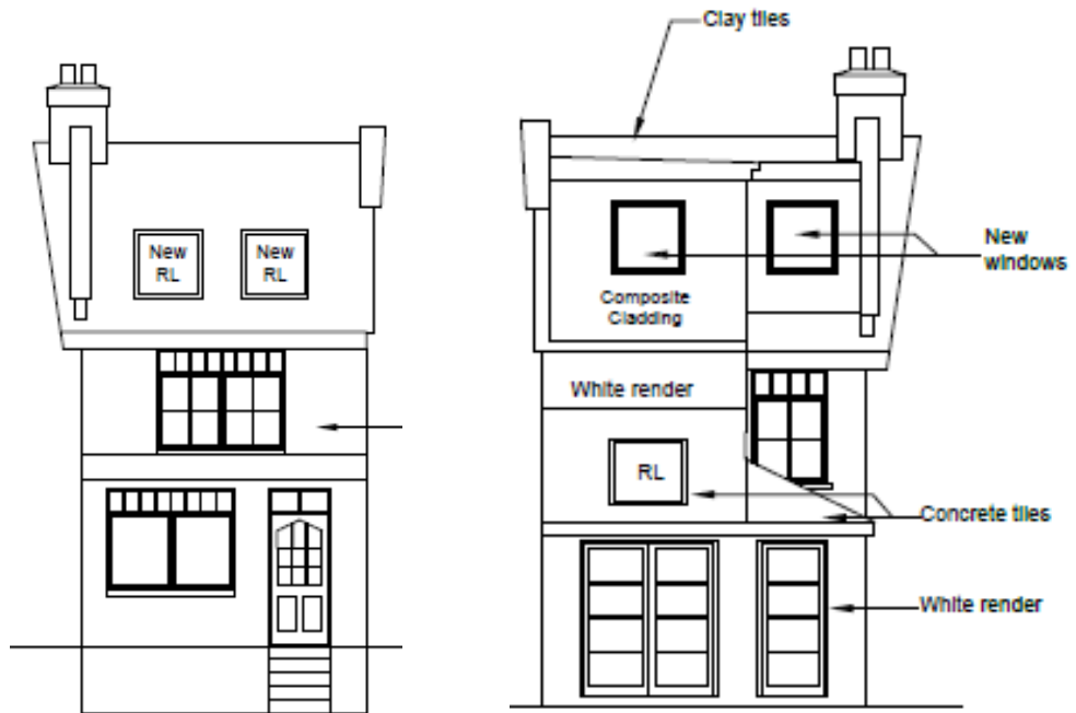
Figure 4 – Existing front and rear elevations
