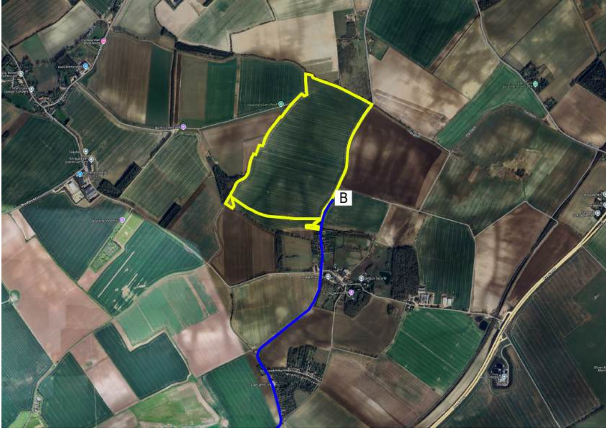
Figure 12: Detailed view of the first section of the construction vehicle route as it exits the site with the aid of a banksman onto Ashwell Road and continues in a southern direction through Bygrave before and continuing onto Ashwell Road. This section shows the bend to the south along Ashwell Road that HGVs would need to negotiate as per the swept path under Figure 6.13. The swept path for the exit movement is also shown under Figure 6.12 (Source: Google Maps).
