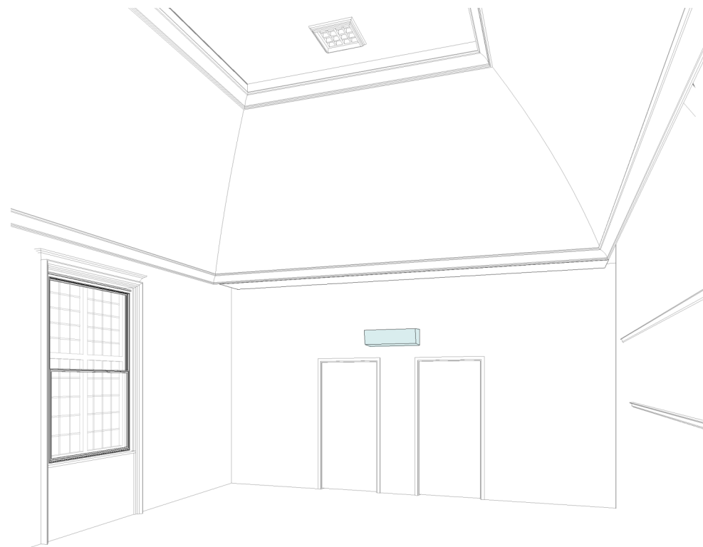
Proposed view of the west of the Lucas Room with Fan Coil Unit Highlighted
