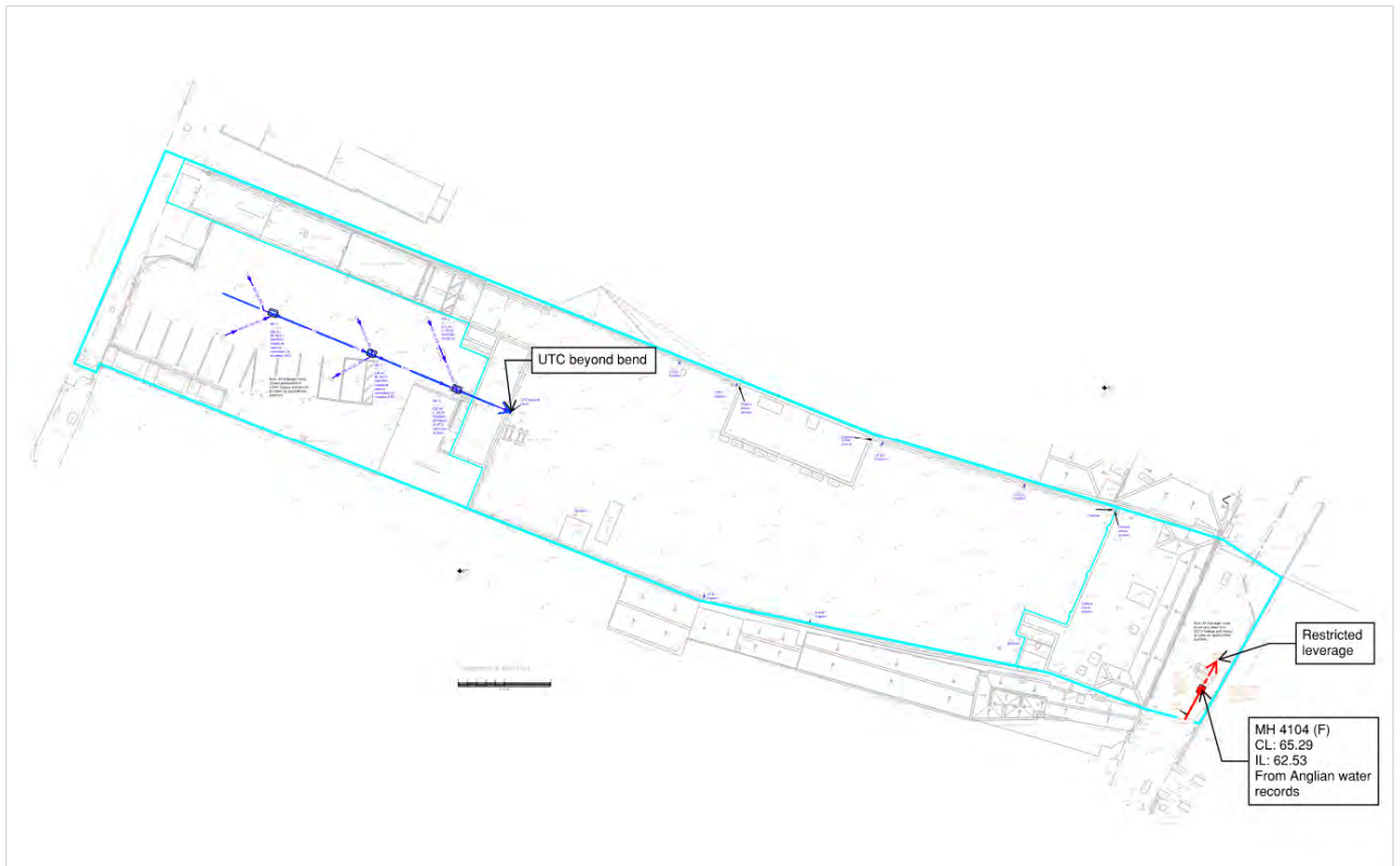
Figure 2.4: Drainage CCTV Survey Layout. (Source: Survey Solutions).
