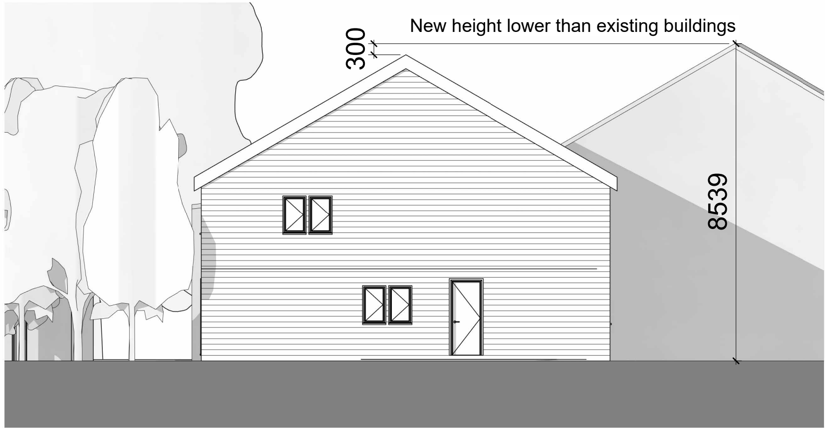
4 Side Elevation - SE - As Proposed 1 : 100
