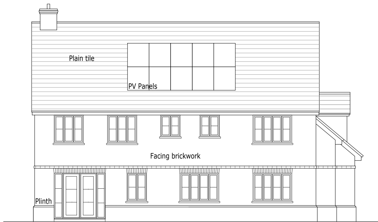
Rear Elevation Solar Panels on Plot 1 ONLY
