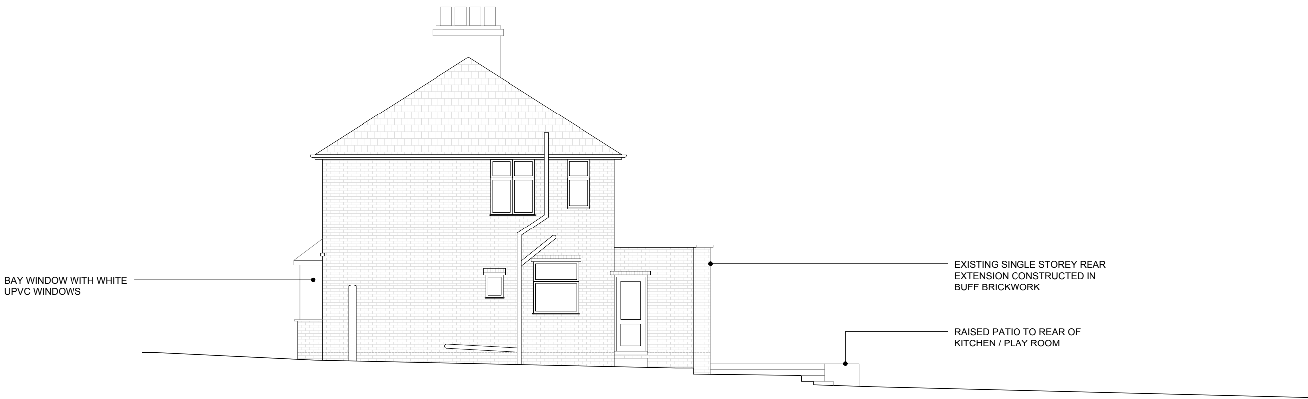
EXISTING SIDE ELEVATION (SOUTH) 1:100 @ A1
