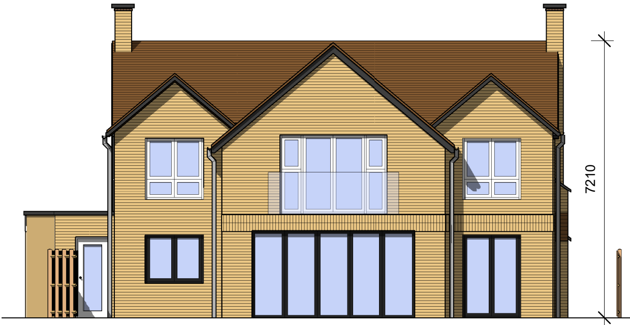
Proposed Rear Elevation 1 : 100
