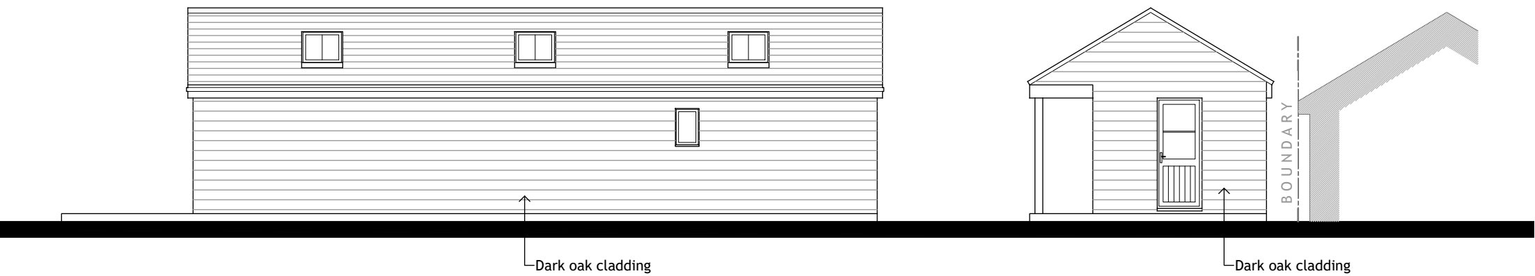
PROPOSED OUTBUILDING - REAR (SOUTH) ELEVATION SCALE 1:100
