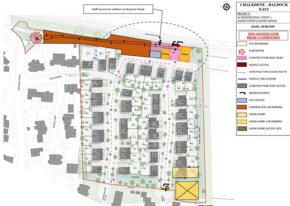
Figure 5b: Site Compound Area for Phase 3 Works
