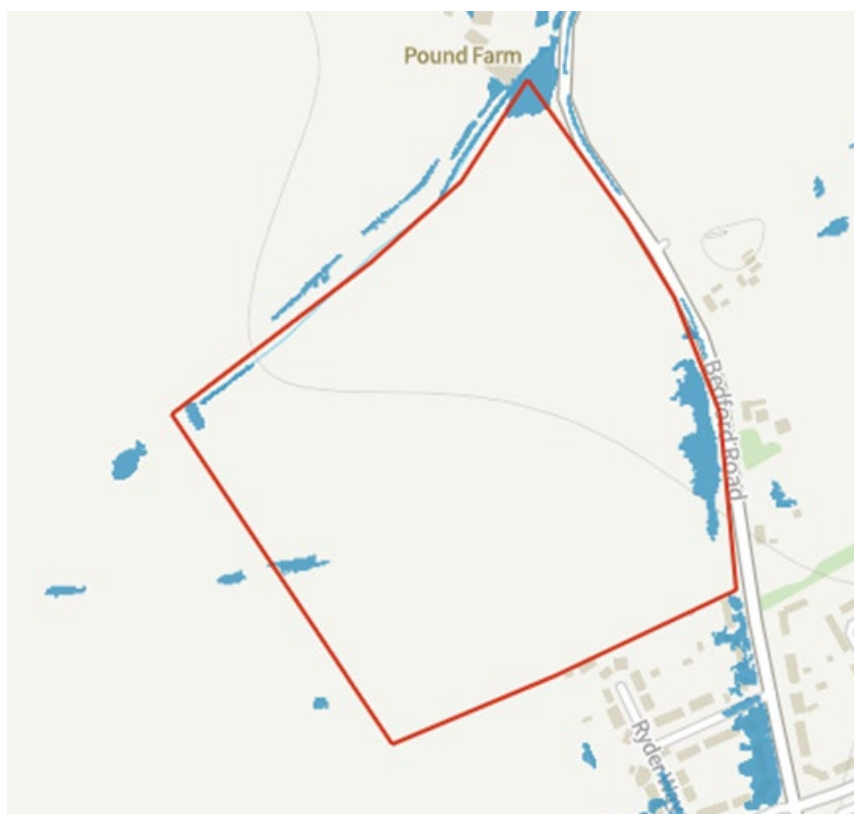
FIGURE 4.1 – EXTENT OF 1 IN 30 YEAR SURFACE WATER FLOODING (HIGH)
