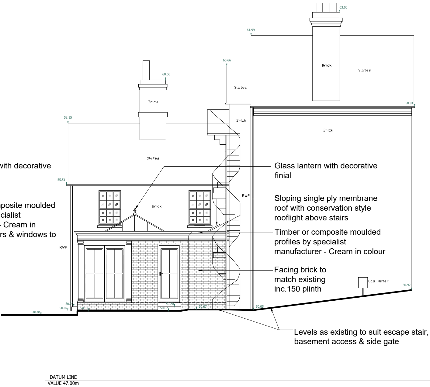
Elevation 2 - Facing West & 30 High Street
