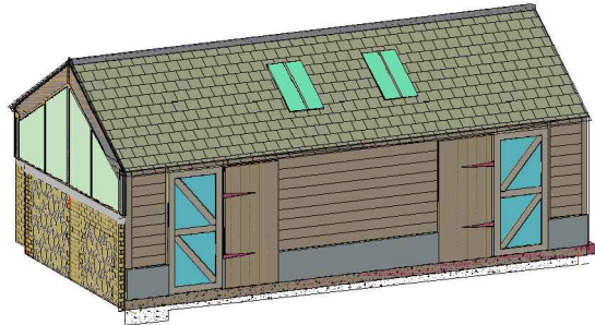
HENHOUSE FRONT ELEVATION showing existing doors retained as shutters with glazed secondary door
