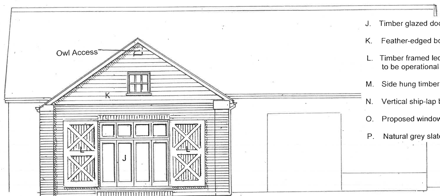
SOUTH WEST ELEVATION
