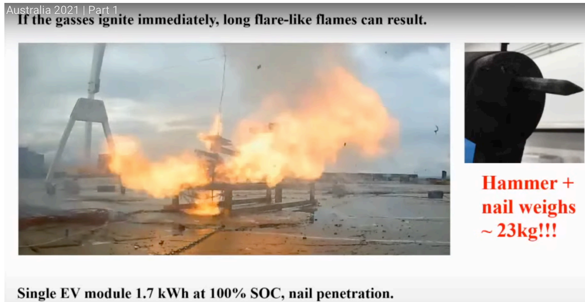
Figure 3 (f). The “long, flare-like flames” last for several minutes as the fire progresses after the initial explosion and ignition
