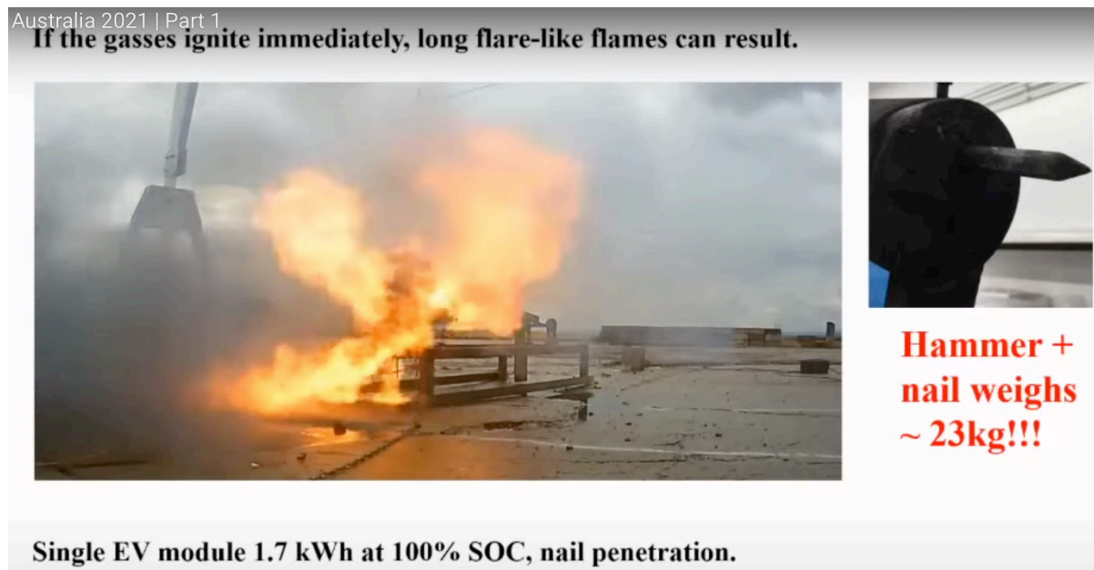
Figure 3 (f). The “long, flare-like flames” last for several minutes as the fire progresses after the initial explosion and ignition
