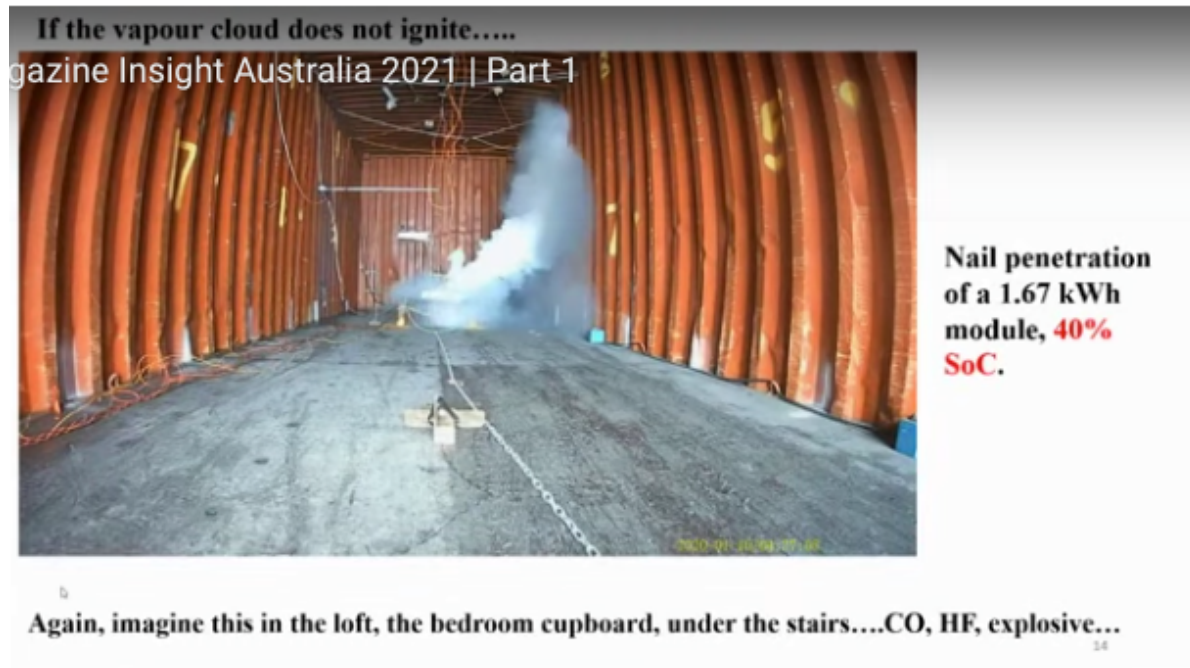
Figure 5 (c): The white vapour cloud follows a fraction of a second later. The light-scattering material creating the opaque white material is likely to be the organic solvents from the cell.
