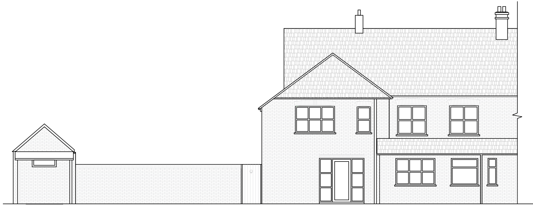
East Elevation— Existing
