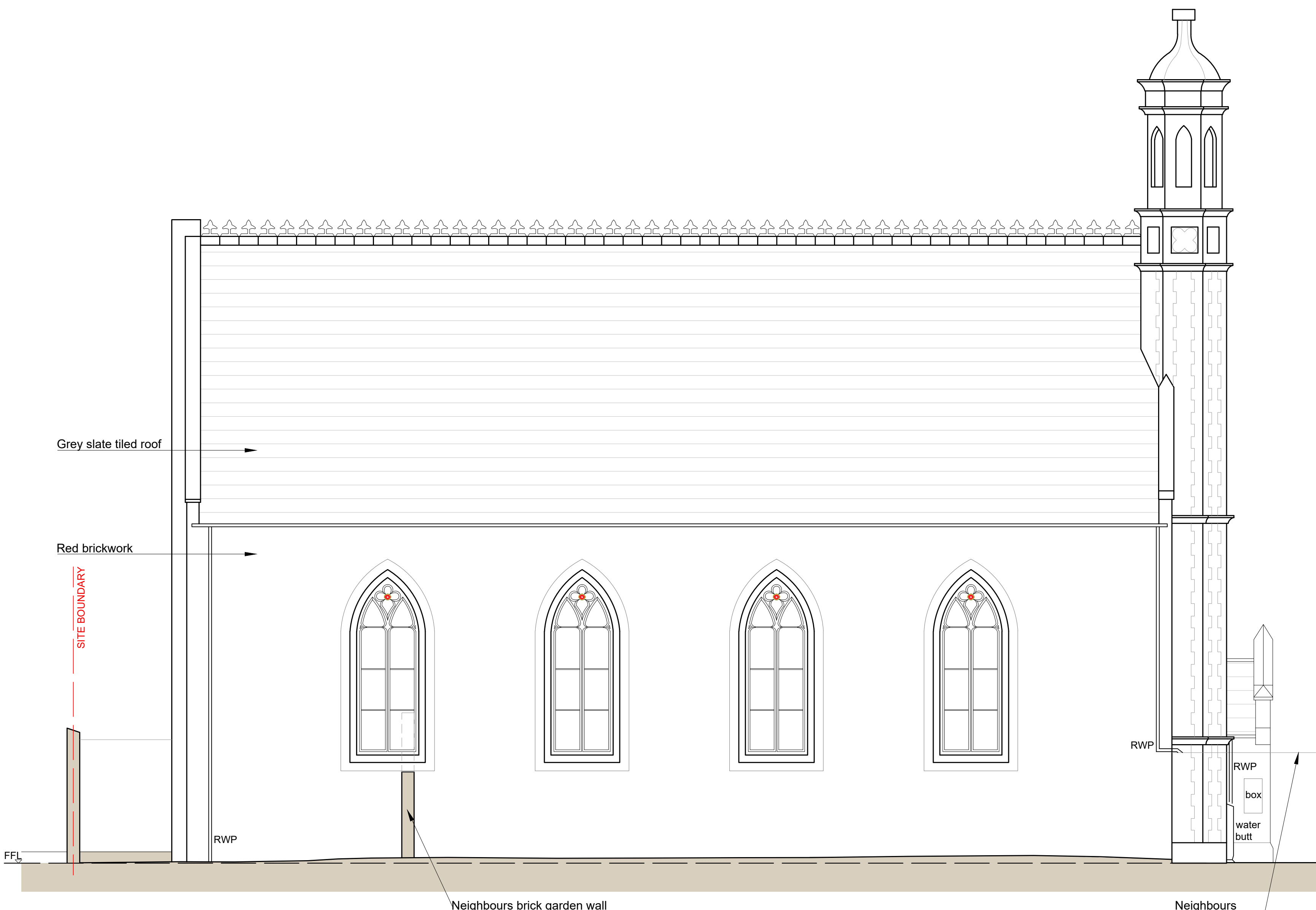
SOUTH WEST (SIDE) ELEVATION
