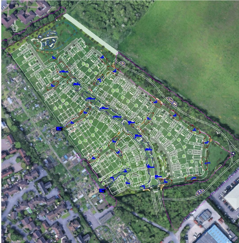
Figure 2: Latest development layout with lighting overlay.
