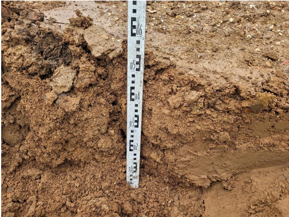
Photo 3: Verified depth of topsoil in plot 5
