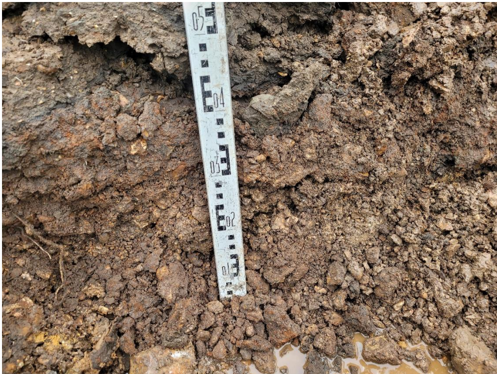
Photo 2: Verified depth of topsoil in plot 6
