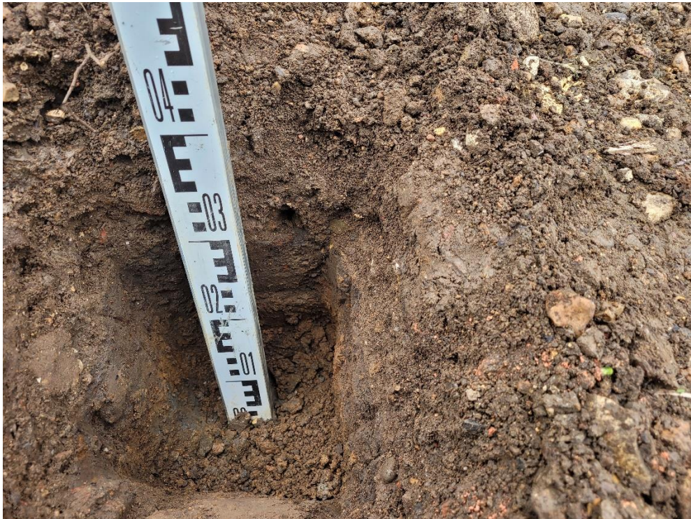
Photo 6: Verified depth of topsoil in plot 4
