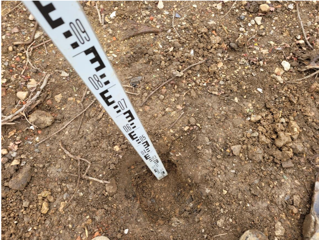
Photo 7: Verified depth of topsoil in plot 1
