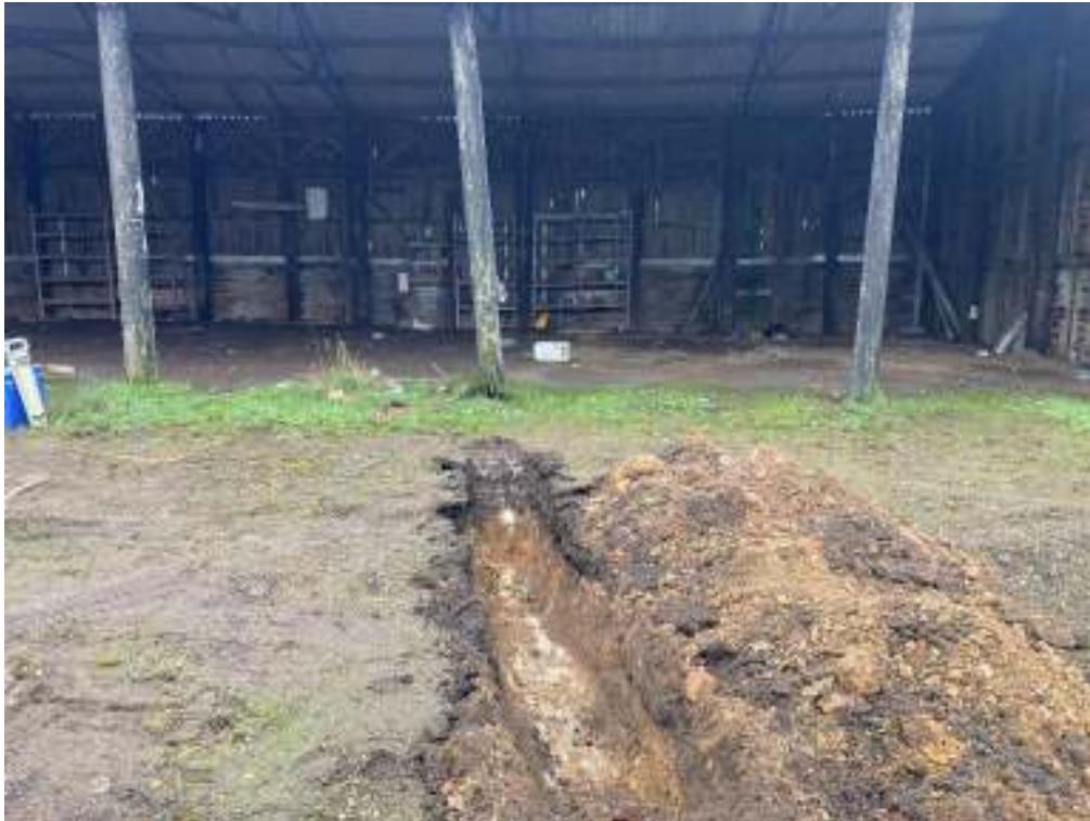
TP1 (Concrete fill at base)
