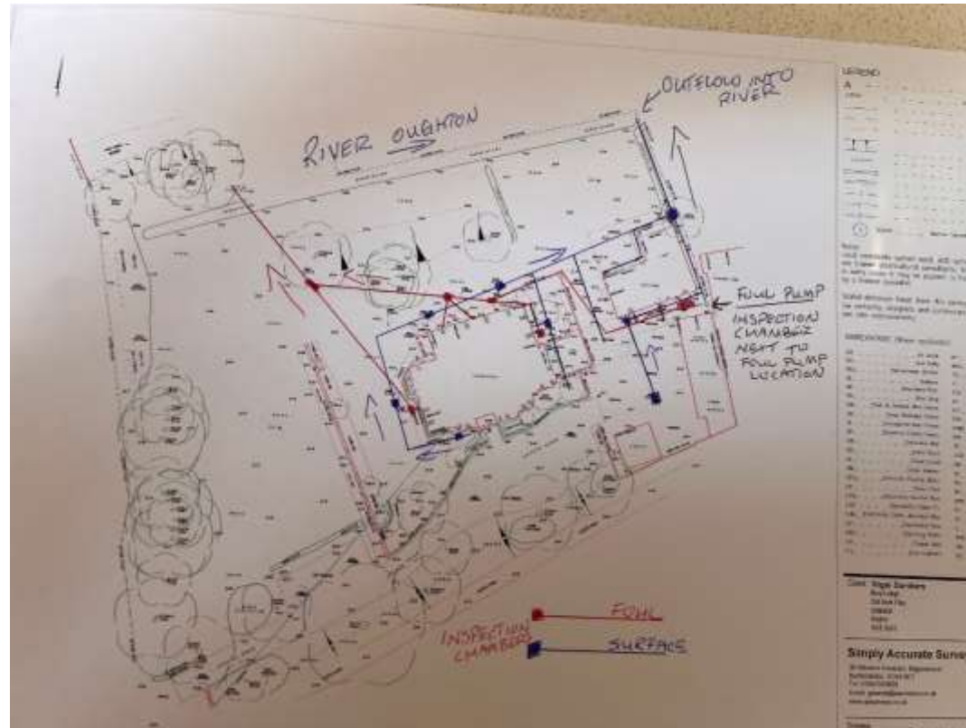
Figure 3 - Private Below Ground Drainage Mark-Up
