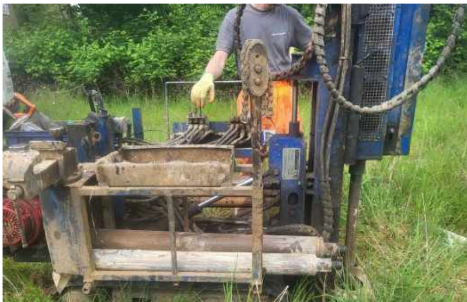
Photo 4 – Window sampling rig operating at BH2
