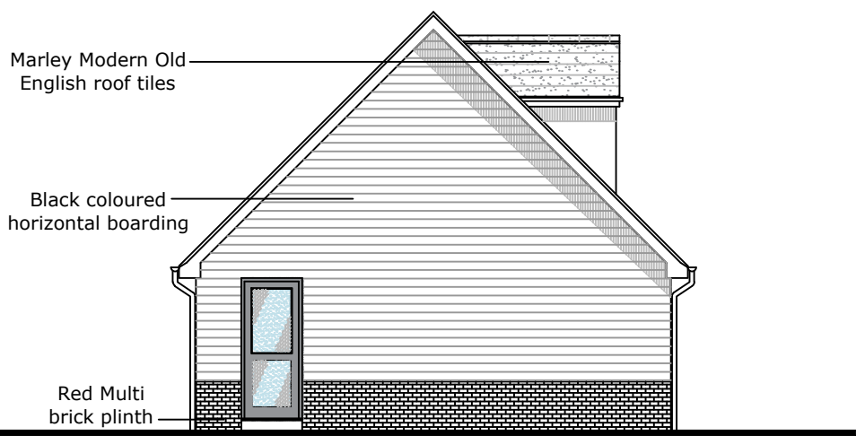
Garage Elevation Side 1:100
