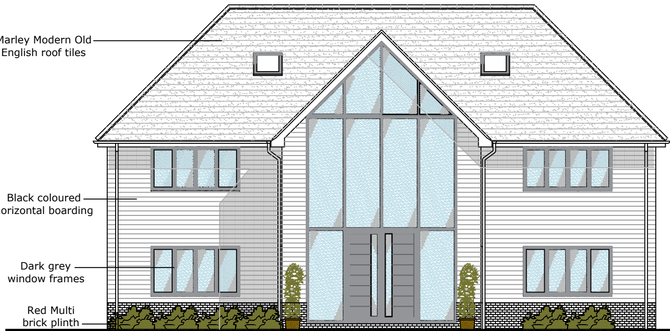
House Elevation Front 1:100
